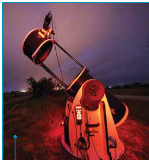
Most of the telescopes used in Senegal and Colombia were 16" Skywatcher instruments, as shown here. Each telescope is shipped in four packing cases. A medium-sized shipping container was required to hold all the cases.
