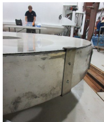
Figure 5: 72-inch Perkins mirror at the DCT coating facility awaiting its new aluminum coating.
