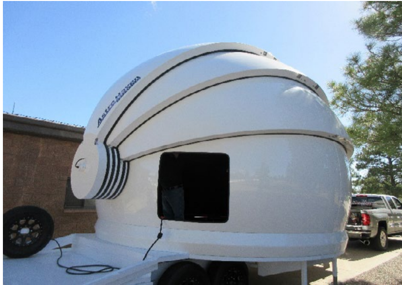
Figure 6: The dome-trailer enclosure system after construction.
