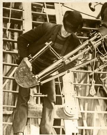
Vesto M. Slipher uses a spectrograph built by John Brashear. Slipher relied on this spectrograph to discover the first evidence of an expanding universe. LOWELL OBSERVATORY ARCHIVES
