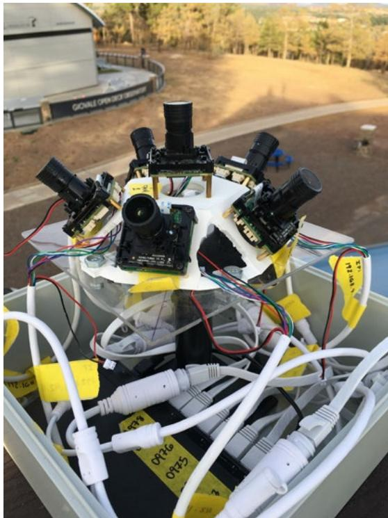
Six-camera LO-CAMS array (sans dome) located on the roof of the Mars Hill instrument shop.
