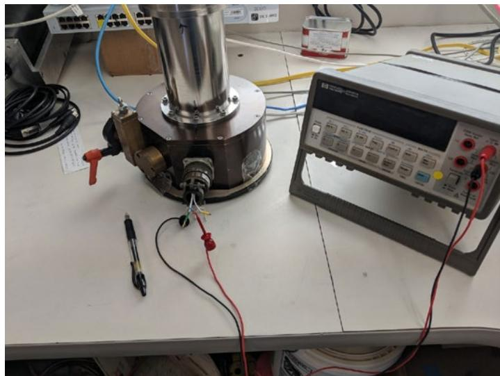
The NASA42 camera being tested after function was restored to its cryogenic system.
