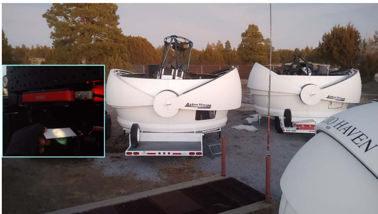
Two of the 1-meter telescopes on-sky for the night for single-aperture robotic telescope use. Inset: an image of the moon on a notecard, in the beam train of the 1-m fast tip-tilt system.
